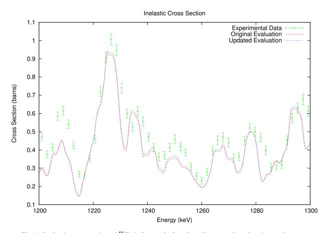
Fig. 4. Inelastic cross section of  $^{56}$ Fe before and after the adjustment based on integral experimental data plotted on top of differential experimental data of Perey, presented with one standard deviation error bars.
