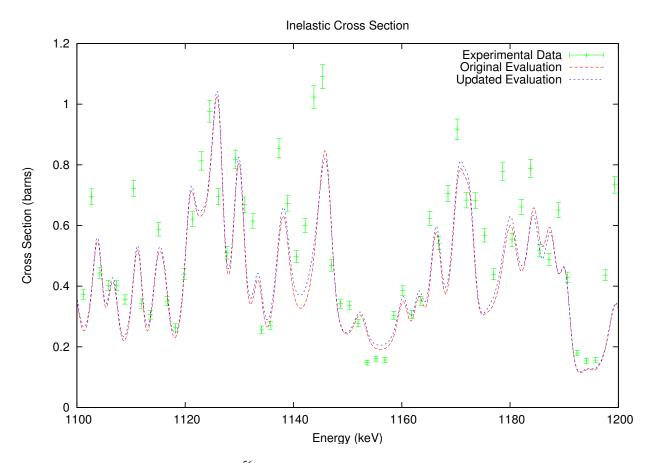
Fig. 3. Inelastic cross section of  $^{56}$ Fe before and after the adjustment based on integral experimental data plotted on top of differential experimental data of Plompen, presented with one standard deviation error bars.
