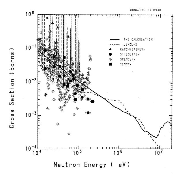
Fig. 17. Radiative capture cross sections.
