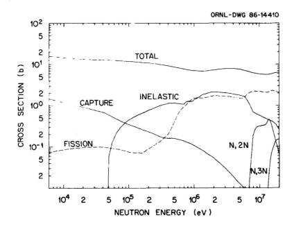
Figure 21. Overview of the present evaluation of  $^{240}\mathrm{Pu}$  above the resolved resonance region.
