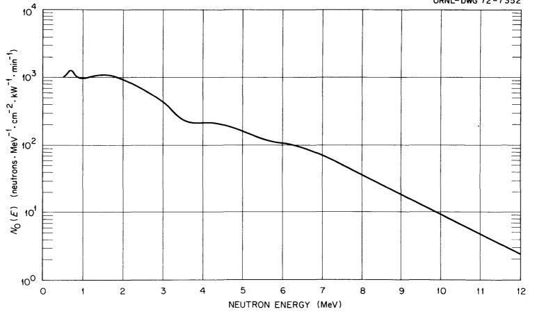
Fig. 3. Source Spectrum for Sodium.
