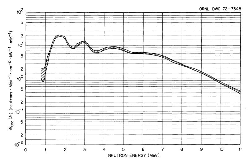
Fig. 2. Transmitted Spectrum Through Sodium.
