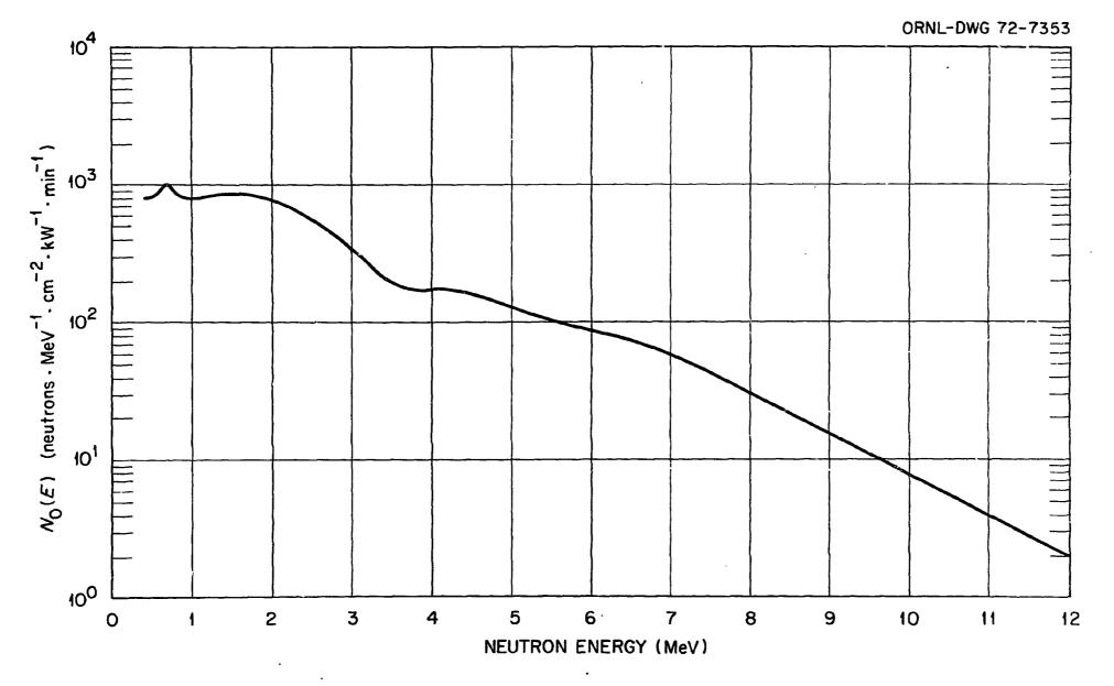
Fig. 3. Source Spectrum for Oxygen.
