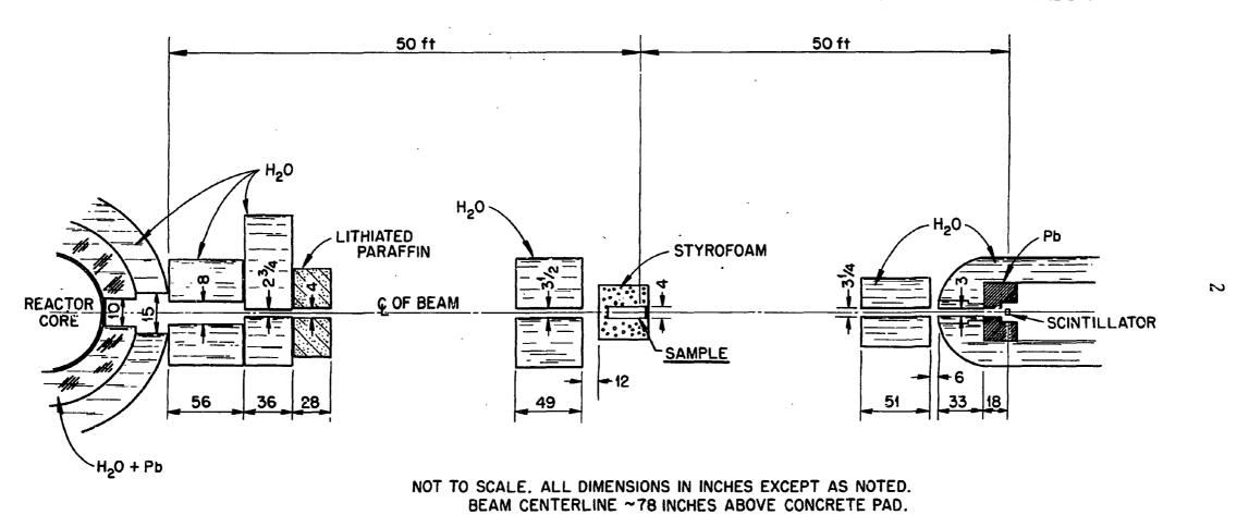
Fig. 1. Schematic of Experimental Arrangement.
