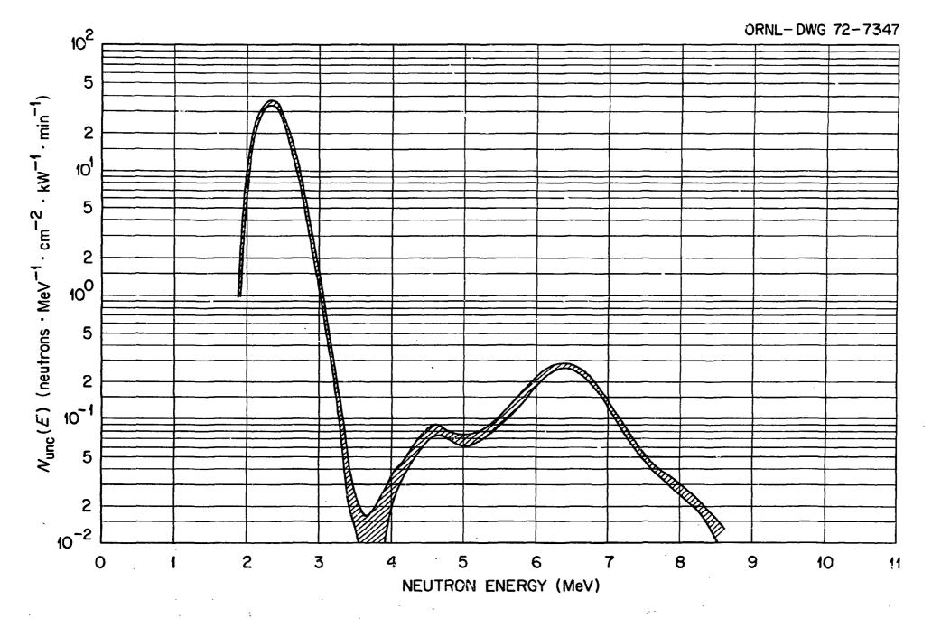
Fig. 2. Transmitted Spectrum Through Oxygen.
