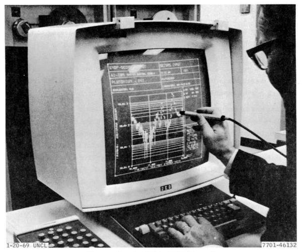
Figure 2. An IBM-2250 Console
